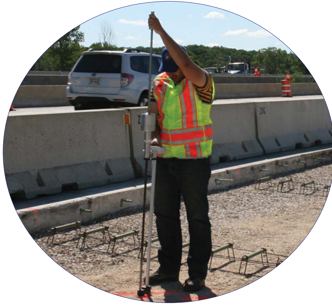
DYNAMIC CONE PENETROMETER TEST
